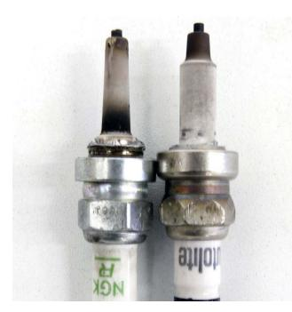
We removed the threads on these two plugs to illustrate heat range. The plug on the left is a hotter heat range than the plug on the right. Note how the hot plug's ceramic has a longer path from the tip of the plug to where the ceramic contacts the plug's shell and then to the head. The colder plug on the right has a much shorter path for the heat to travel; it pulls heat more efficiently from the plug tip so it will not burn off carbon as easily.
