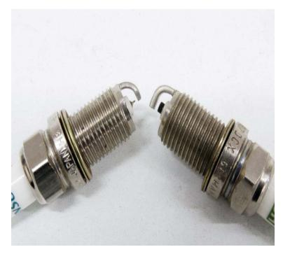
This compares an extended-nose plug (left) to a standard-reach plug (right). Note how much longer the extended-reach plug's ground strap is compared to the standard-reach. For street engines, the extended-nose is good for part-throttle efficiency. The shortreach is far better for high output engines where the longer ground strap could get hot enough to cause preianition.
