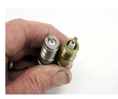
The addition of precious metal in the center electrode has nothing to do with the heat range of a spark plug. The heat range is designed into the relationship of the ceramic to the plug body. The plug on the left is a cold plug with a shallow ceramic depth. The plug on the right is a much hotter plug with the ceramic connecting with the outer shell much deeper.
