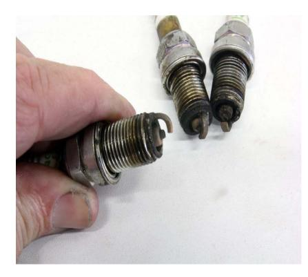
This is a used plug from a small-block Chevy that had started out with roughly 0.040-inch gap and the copper core has worn to 0.050-inch. A wider gap increases the load on the ignition system, demanding higher voltage. Replacing this with a fine-wire plug would allow running a decent plug gap and still offer the potential for improved combustion.
