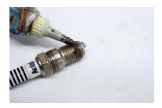
Spark plug companies don't recommend anti-seize on threads because it lowers the torque required to install the plug. Torqueing the plugs to the published spec with anti-seize over torques the plug which potentially could break the internal seal between the insulator and the shell, creating a leak path. So it's best to install spark plugs dry.
